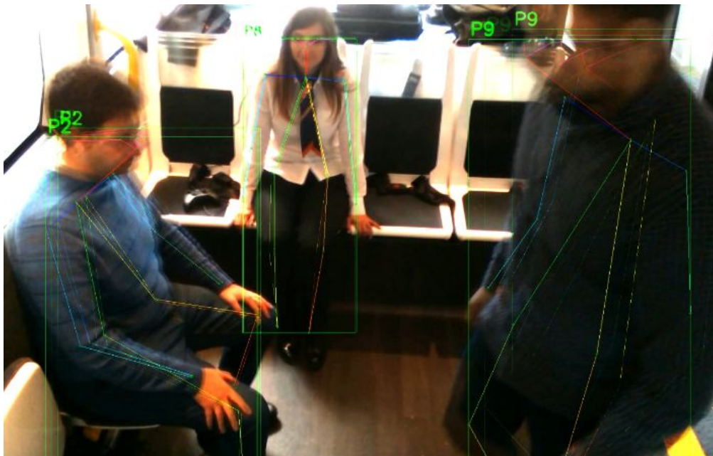
Figure 4. Skeleton matching across two different frames (blended)
