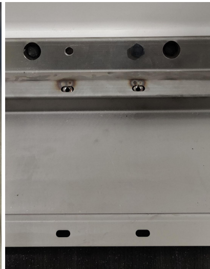
Figure 3.15, left: Bolts used for attaching anchor construction to the glass fibre construction.
