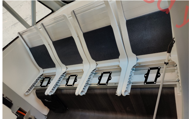
Figure 3.10: Bottom of seats removed. Placement of original seat belt attachers shown in black
